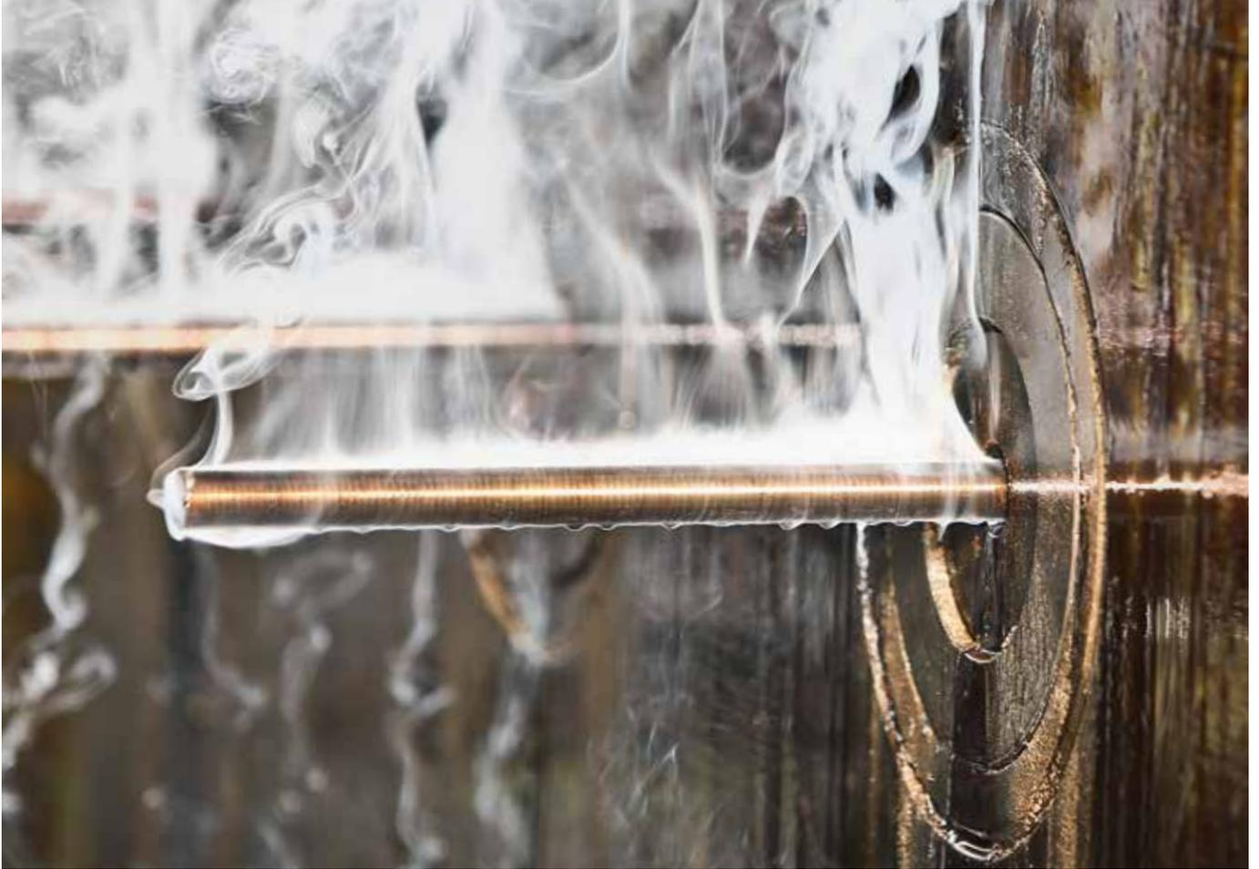
Drawing unit at Steeltec.
