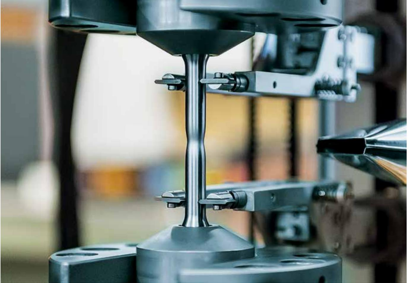
The mechanical properties of our products are determined in tensile tests.
